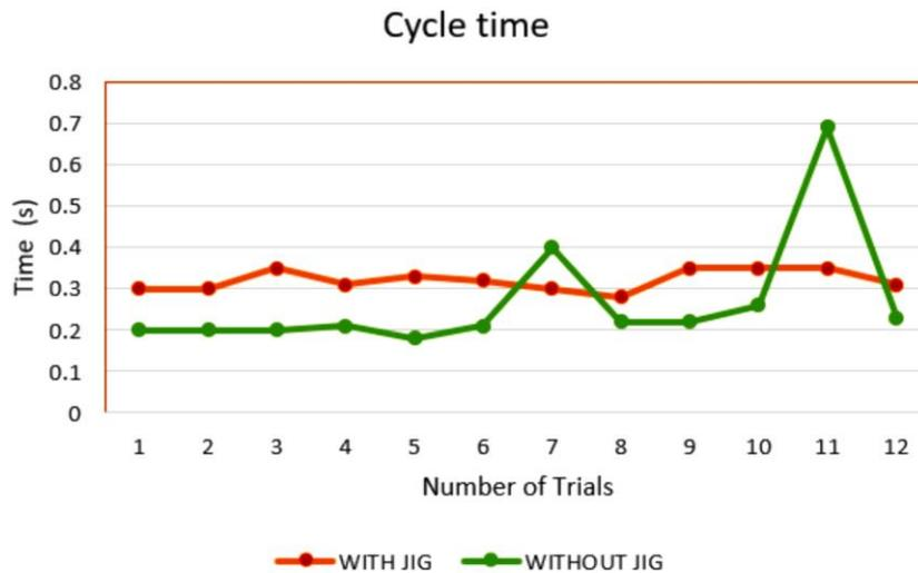
**Fig. 7. Cycle time study for SSW process with and without the Poka yoke jig.**
