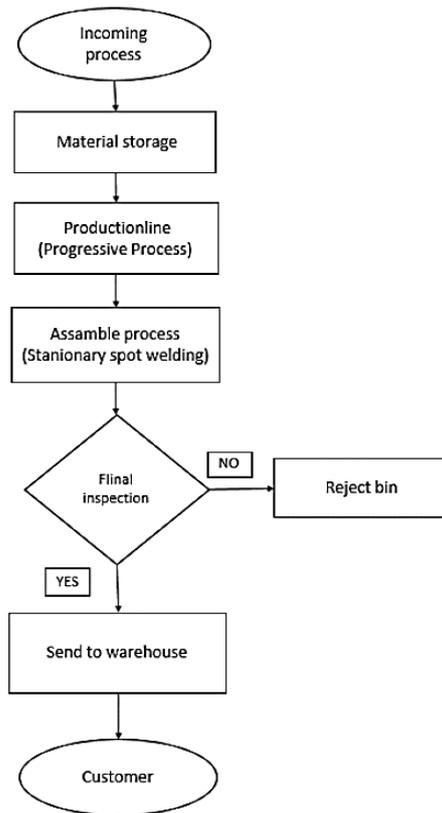
**Fig. 4. Flow chart of production process flow.**
