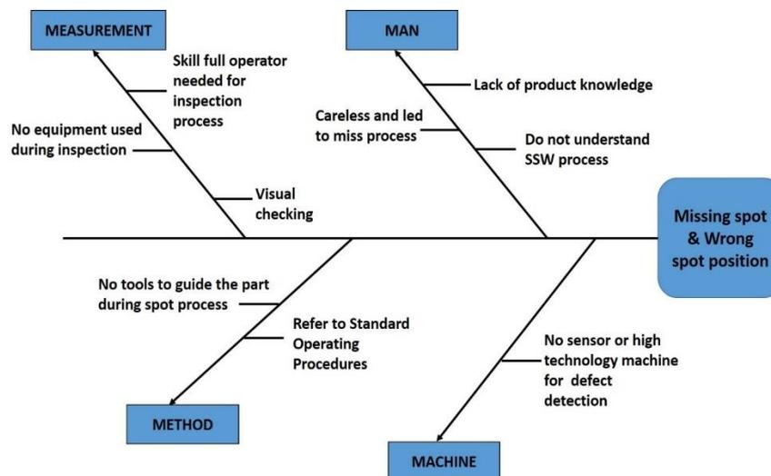
**Fig. 6. Cause and effect diagram for defects; miss spot and wrong spot position.**
