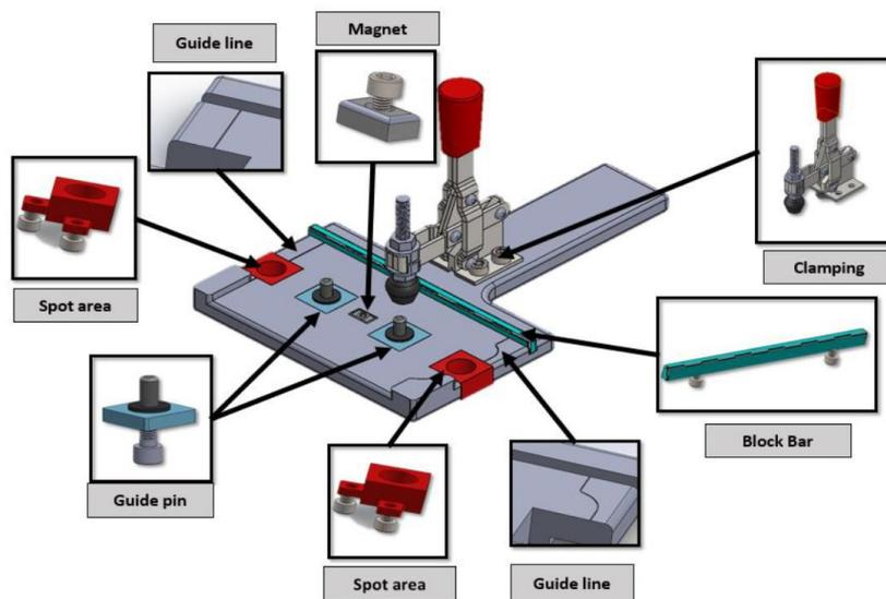
**Fig. 9. Final concept design of Poka yoke jig for SSW process in this project.**
