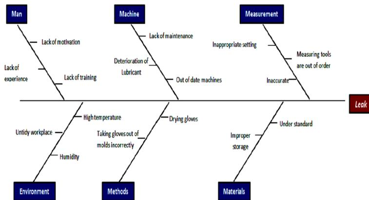
Fig. 3. Example of cause and effect diagram analysis for SSW issue [8].
