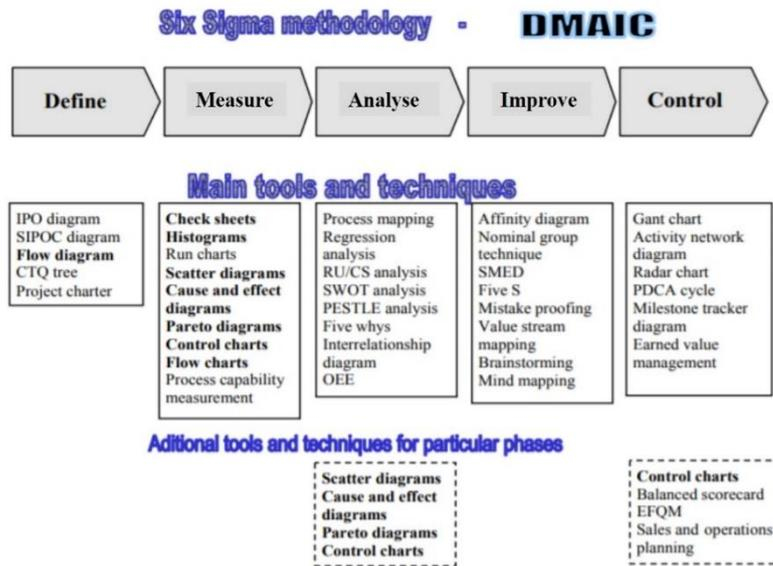
**Fig. 1. DMAIC the Six Sigma methodology.**
