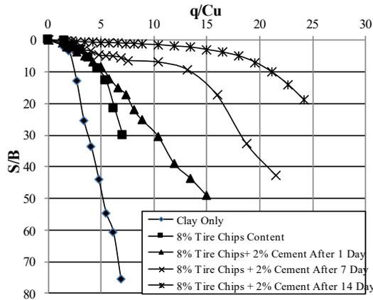
**Fig. 9.  $q/C_u$  Variation with  $S/B$  for treated soil by 8% tire chips content and cement with time ( $D= 0.25B$ ).**
