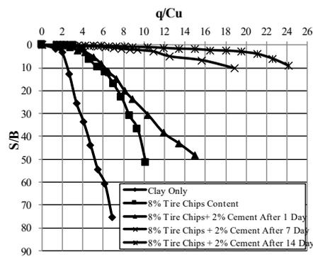
**Fig. 12.  $q/C_u$  Variation with  $S/B$  for treated soil by 8% tire chips content and cement with time ( $D= 0.5B$ ).**
