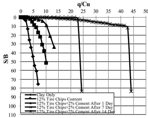
Fig. 13.  $q/C_u$  Variation with  $S/B$  for treated soil by 12% tire chips content and cement with time ( $D= 0.5B$ ).
