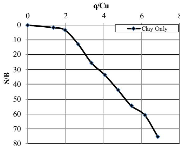
**Fig. 7. q/Cu variation with S/B for untreated soil.**
