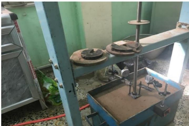
**Fig. 3. Loading assembly and steel container.**
