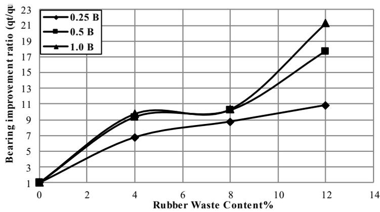
**Fig. 19. Bearing improvement ratio versus rubber waste content after a 14-day curing.**
