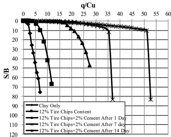
Fig. 16.  $q/C_u$  Variation with  $S/B$  for treated soil by 12% tire chips content and cement with time ( $D= 1B$ ).
