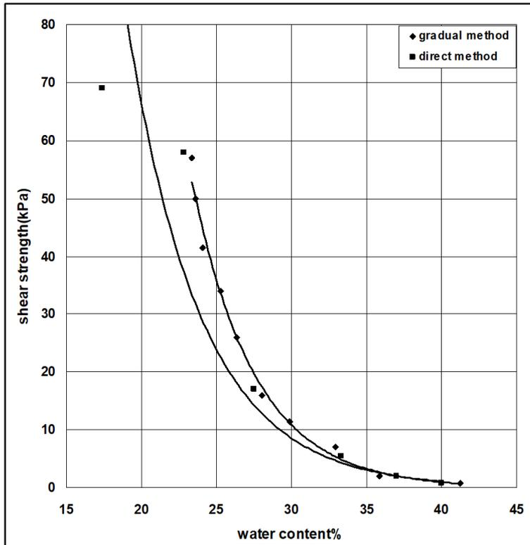
Fig. 5. Undrained shear strength variation with water content.
