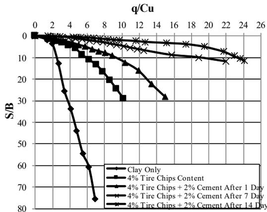
Fig. 14.  $q/C_u$  Variation with  $S/B$  for treated soil by 4% tire chips content and cement with time ( $D= 1B$ ).
