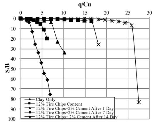
**Fig. 10.  $q/C_u$  Variation with  $S/B$  for treated soil by 12% tire chips content and cement with time ( $D= 0.25B$ ).**
