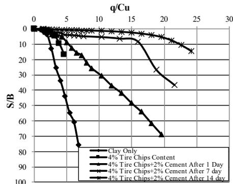
**Fig. 11.  $q/C_u$  Variation with  $S/B$  for treated soil by 4% tire chips content and cement with time ( $D= 0.5B$ ).**
