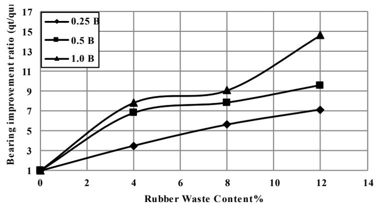
**Fig. 18. Bearing improvement ratio versus rubber waste content after 7-day curing.**
