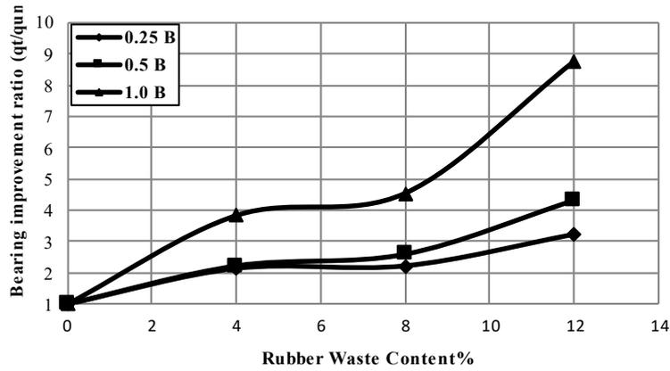
**Fig. 17. Bearing improvement ratio versus rubber waste content after 1-day curing.**
