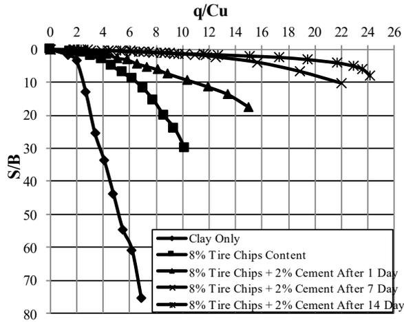
Fig. 15.  $q/C_u$  Variation with  $S/B$  for treated soil by 8% tire chips content and cement with time ( $D= 1B$ ).
