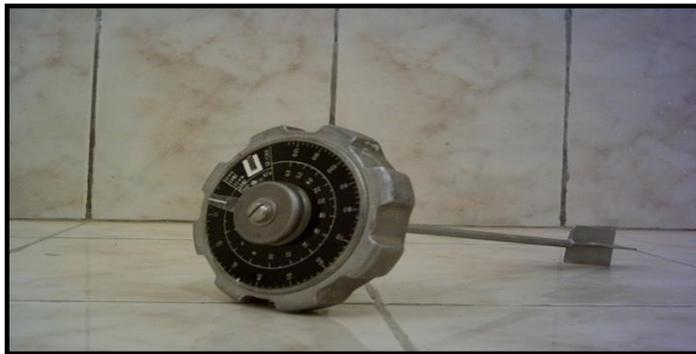
**Fig. 4. Portable vane shear device.**
