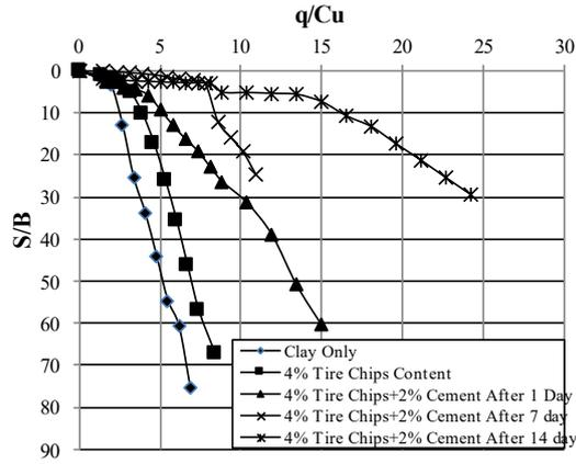
**Fig. 8.  $q/C_u$  Variation with  $S/B$  for treated soil by 4% tire chips content and cement with time ( $D= 0.25B$ ).**
