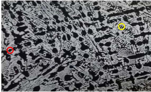
Fig. 6. A microscopic image of nickel-chrome alloy white cast iron material based on ASTM A532 Type I standard. The Red circle indicates the chrome carbide, and the yellow circle indicates the martensite.
