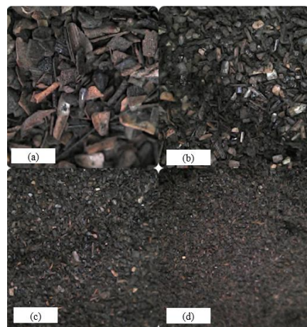
Fig. 5. Microscope observation surface of specimens containing rice husk particles in the brake pad. Figures were classified as (a) 79, (b) 89, (c) 125 and (d) 250 \mu\text{m} .
