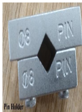
Fig. 4. Pin holder (For 8 mm pin).
