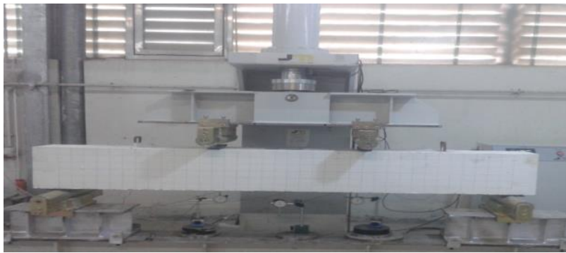
Fig. 7. The beam location in the loading test machines.
