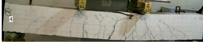
Fig. 13. Cracking pattern of beam B4.
