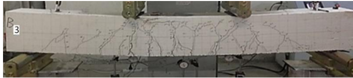
Fig. 12. Cracking pattern of beam B3.
