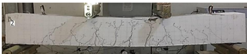
Fig. 11. Cracking pattern of beam B2.
