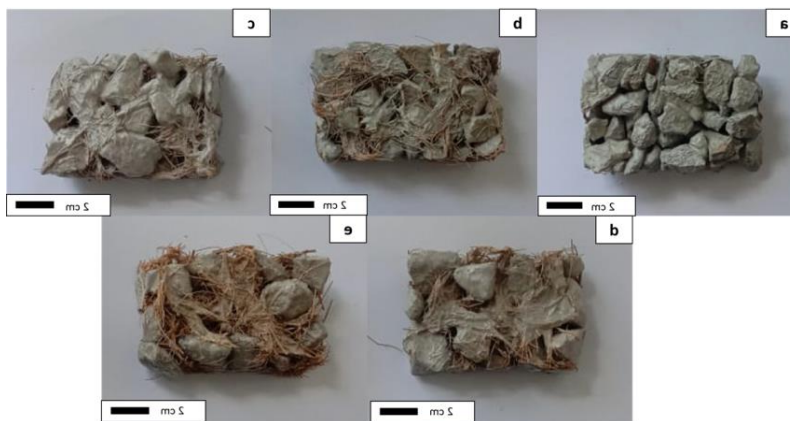
Fig. 2. The physical appearance of porous concrete with various admixtures containing coconut shells and coconut fiber.
