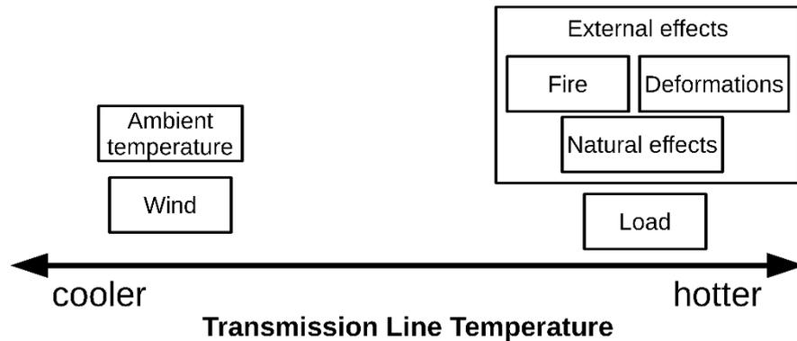
Fig. 1. External factors affecting the transmission line temperature.
