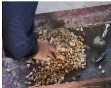
(b). 25% of the water is used to wet the aggregate
