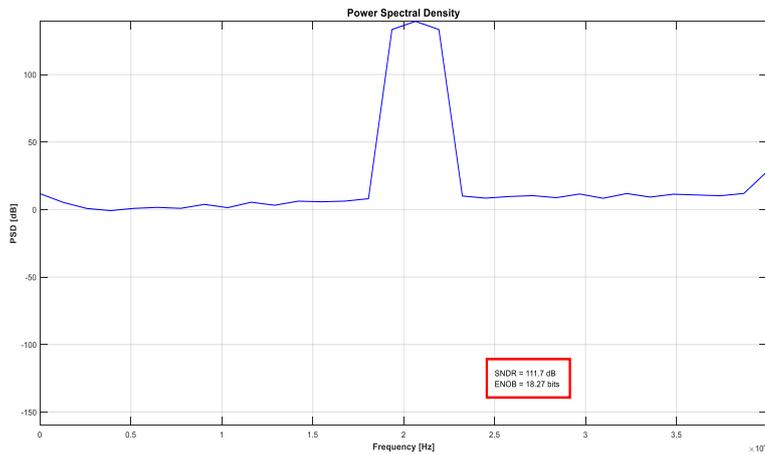
**Fig. 9.** PSD for the first FIR Filter output signal spectrum by OSR of 2.
