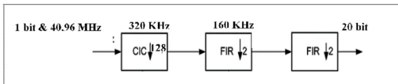
**Fig. 5. Decimation filters architecture.**
