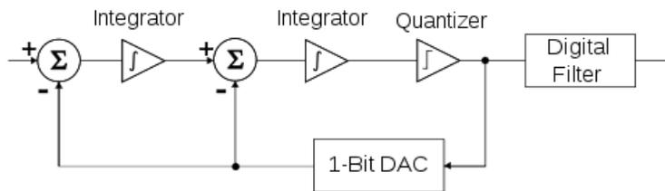
**Fig. 4. Design of  $\Sigma\Delta$  analog to digital system.**
