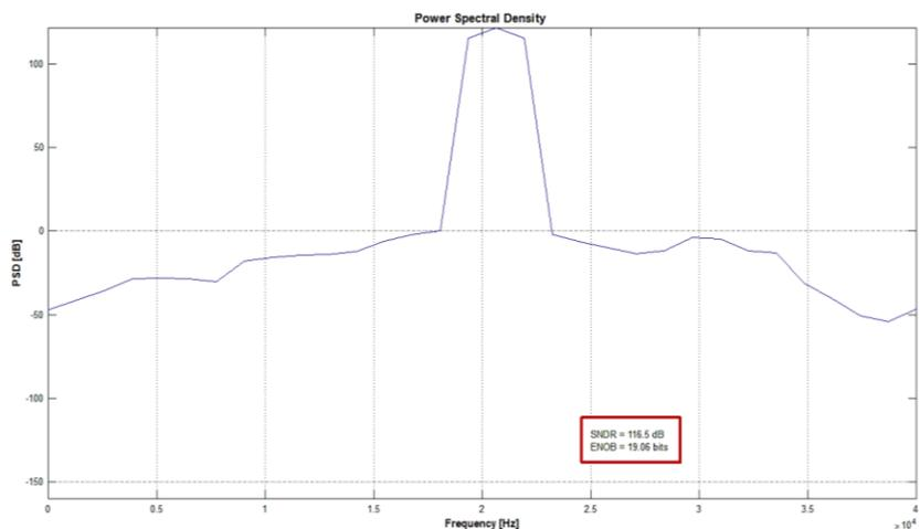
Fig. 10.  $\Sigma\Delta$  Output power spectral density (PSD) at 40.96 MHz.
