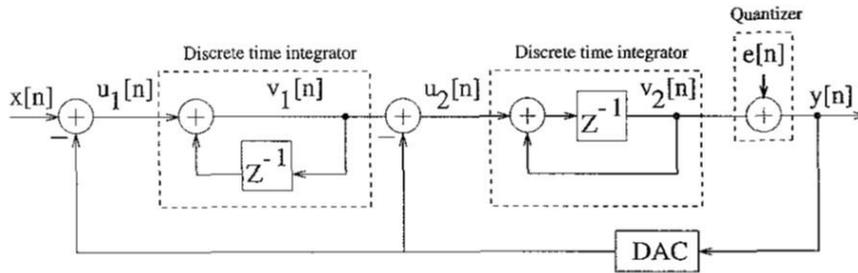
Fig. 2. Second order  $\Sigma\Delta$  modulator [7].
