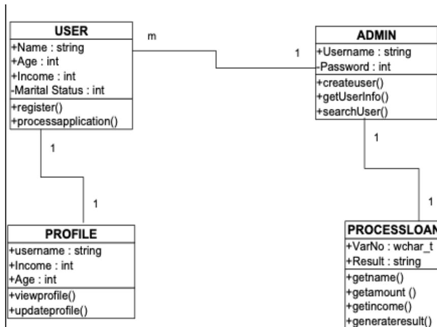
Fig. 4. Class diagram of a loan prediction system.
