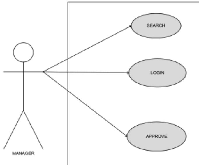
Fig. 2. A use case diagram for a manager of a loan prediction system.
