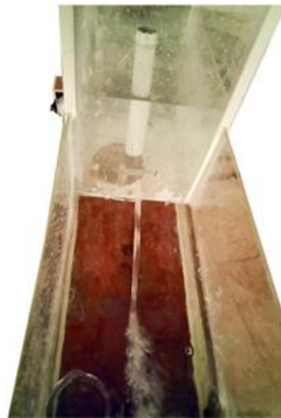
Fig. 2. Opening: d = 12.7 mm and L = 4 mm.
