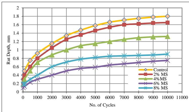
Fig. 19. Impact of the addition of the MS on rutting depth.
