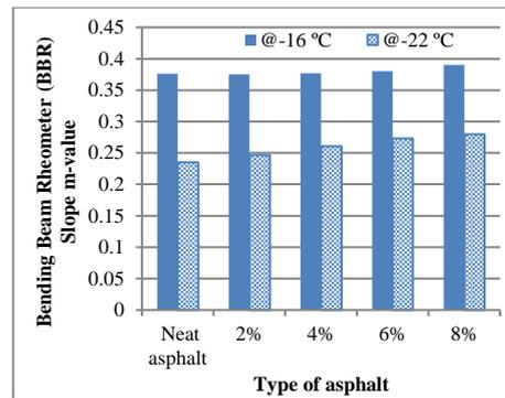
**Fig. 13. Effects of MS ratios on BBR values for PAV binder.**
