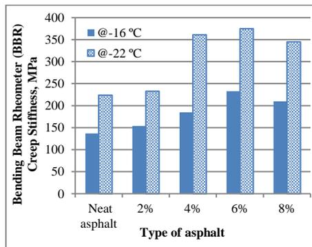
Fig. 12. Effects of NS ratios on BBR values for PAV binder.
