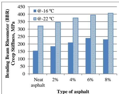
Fig. 11. Effects of MS ratios on BBR values for PAV binder.
