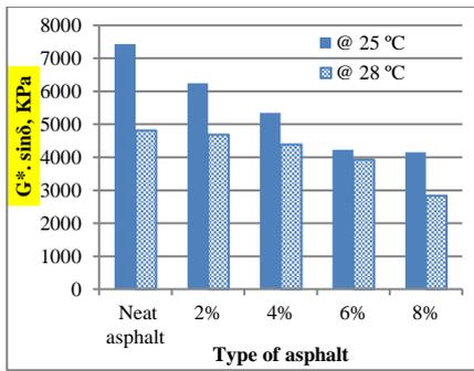
Fig. 9. Effects of NS ratios on DSR values after PAV test.
