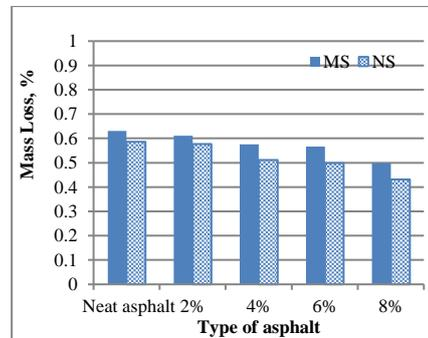
Fig. 10. Effects of MS and NS ratios on mass losing.
