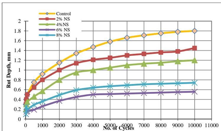
Fig. 20. Impact of the addition of the NS on the rutting depth.
