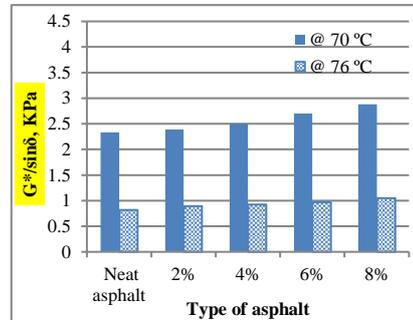
Fig. 4. Effects of MS ratios on DSR values for original binder.
