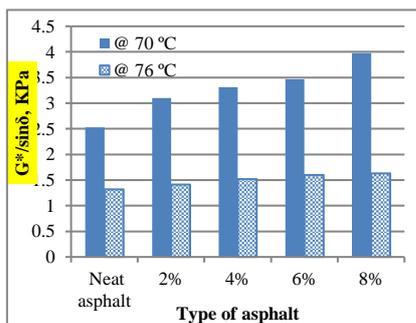
Fig. 7. Effects of NS ratios on DSR values after RTFO test.
