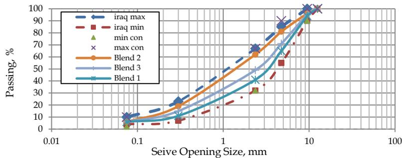
**Fig. 1. Trail selected aggregate gradation blends.**
