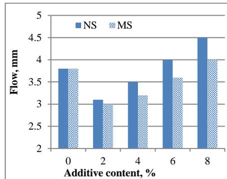
Fig. 16. Impact of the addition of the MS and NS on Marshall flow at OAC.
