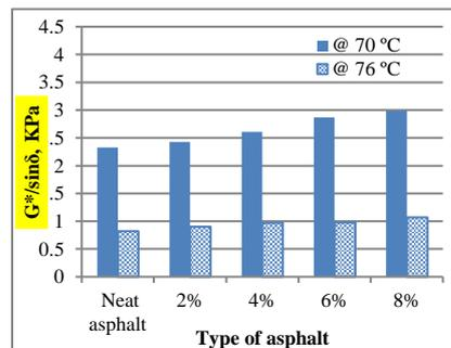
Fig. 5. Effects of NS ratios on DSR values for original binder.
