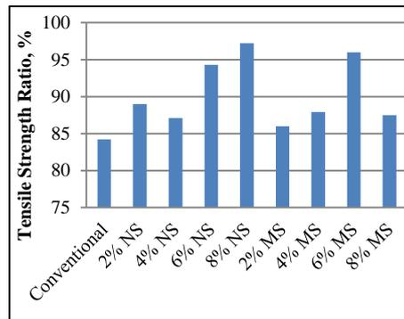
Fig. 18. TSR values for each mixture.
