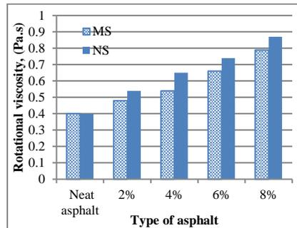
Fig. 3. Impact of type of asphalt on rotational viscosity at 135°C.
