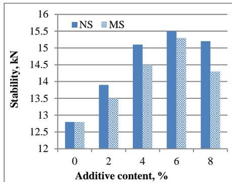
Fig. 15. Impact of the addition of the MS and NS on Marshall stability at OAC.
