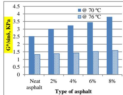
Fig. 6. Effects of MS ratios on DSR values after RTFO test.
