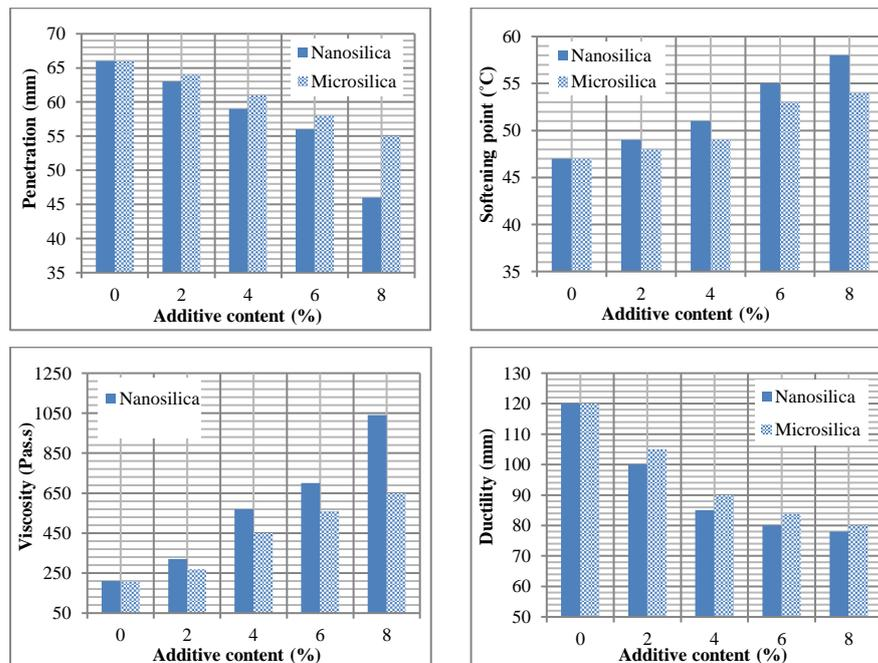
Fig. 2. Physical laboratory tests of modified asphalt.
