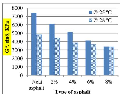
Fig. 8. Effects of MS ratios on DSR values after PAV test.
