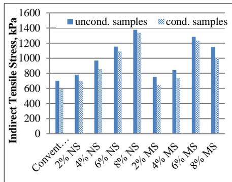
Fig. 17. ITS values for unconditioned and conditioned for each mixture.
