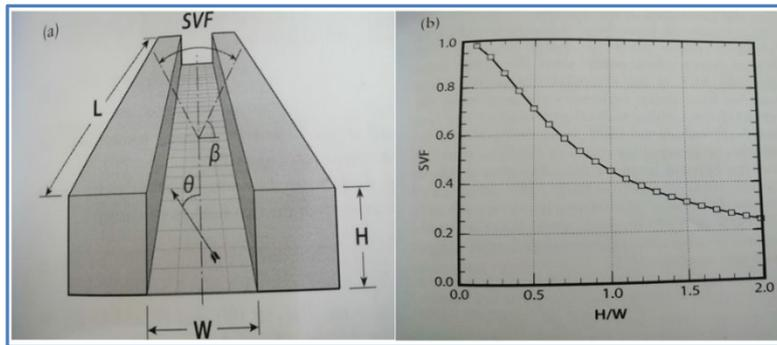
**Fig. 1. Schematic view of a symmetrical urban canyon and its geometric descriptors (a) and sky view factor (SVF) as a function of canyon aspect ratio (H/W) [1].**
