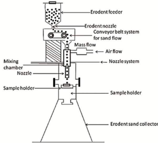
Fig. 3. Air jet erosion test rig [9].
