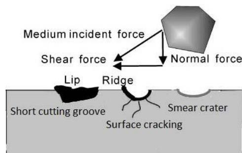
**Fig. 9. Schematic mechanism of erosion at variant impingement angle.**
