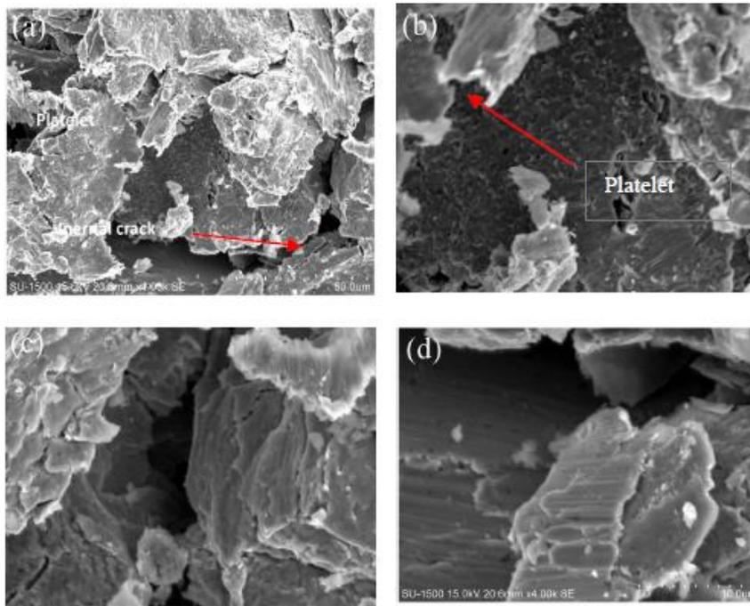
**Fig. 8. SEM micrographs of eroded surfaces at 90° impingement of WC- 11Co-2Cr fine powder size 27.5 μm (a) 1000X, (b) 2000X, (c) 3000x and (d) 4000X.**
