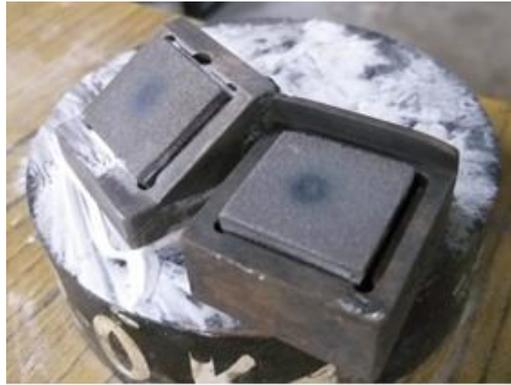
**Fig. 5. Eroded coating specimens.**
