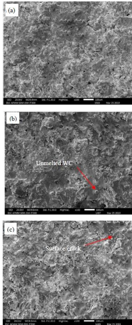
**Fig. 2. SEM images of tungsten carbide (WC-Co-Cr) coatings deposited on base material Inconel-601. (a) WC-8Co-2Cr, (b) WC-11Co-2Cr, (c) WC-14Co-2Cr.**
