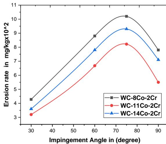
Fig. 4. Comparison of erosion rate vs. impingement angle.
