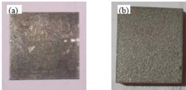
**Fig. 1. (a) Base metal Inconel 601, (b) WC-8Co-2Cr coated specimen.**
