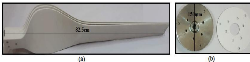
Fig. 2. Blades of wind turbine adopted in this study (a) blade front view, (b) the blades hub.
