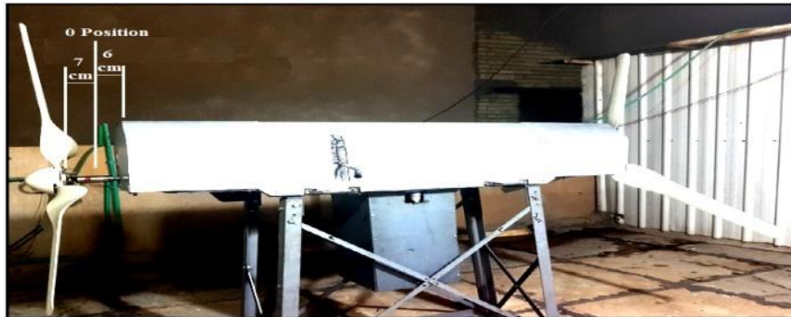
Fig. 15. The distance between the front and rear blades changing about 7 cm.
