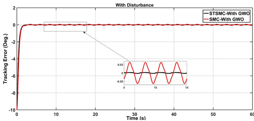
**Fig. 12. Behavior of tracking errors with gust wind uncertainty.**
