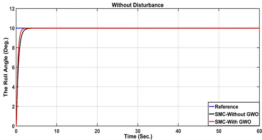
Fig. 6. Behavior of roll angle SMC.
