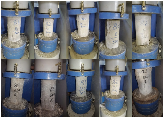
Fig. 12. Strength in compression test for cylinder for several heating degrees and cooling methods.
