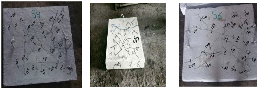
(a) Failure mode of S4. (b) Failure mode of S5. (c) Failure mode of S6. Fig. 13. Failure modes of group B.
