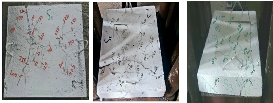
(a) Failure mode of S1. (b) Failure mode of S2. (c) Failure mode of S3. Fig. 12. Failure modes of group A.
