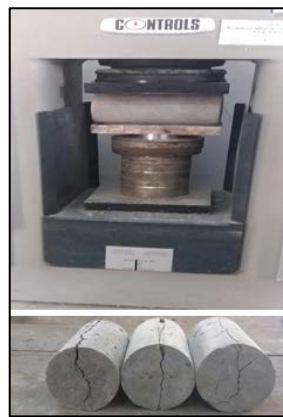
Fig. 3. Splitting tensile strength test.
