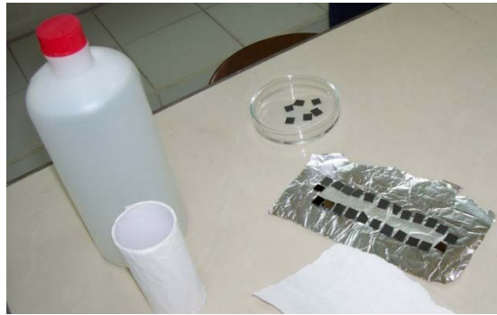
Fig. 2. Pt (200) / SiO 2 / Si (100) and p-type Si (100) substrates.
