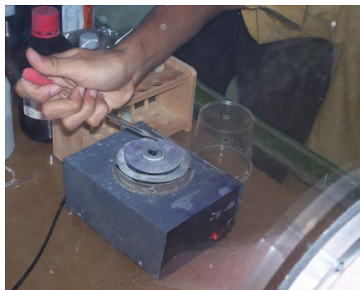
Fig. 3. Thin-film growth on the substrate.
