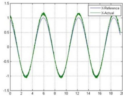
**Fig. 9. Reference and response in x-direction when tracking a circle.**
