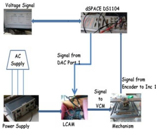
**Fig. 6. Experimental setup with integration of XY mechanism with dSPACE DS1104.**
