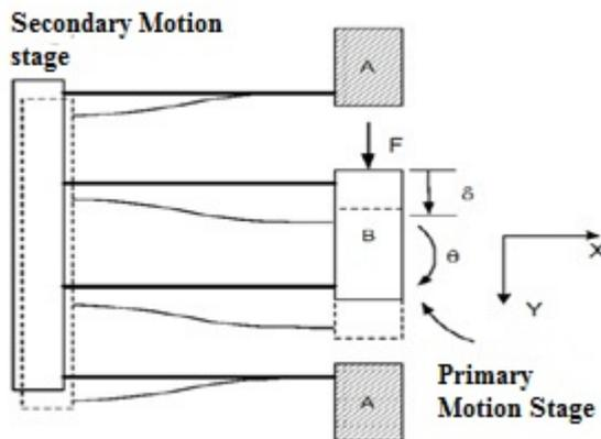
Fig. 4. Double parallelogram flexure.
