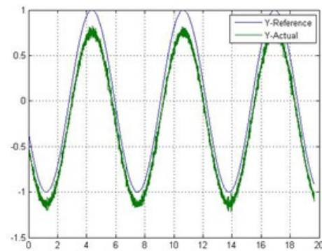
**Fig. 10. Reference and response in y-direction when tracking a circle.**
