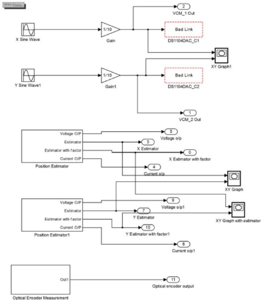
**Fig. 8. The Simulink model for running under real-time work environment in dSPACE.**
