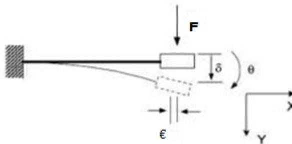
Fig. 2. Cantilever beam with end point load.
