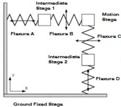
Fig. 1. Topology of flexure mechanism.
