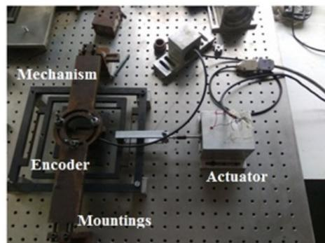
**Fig. 7. The Experimental platform.**
