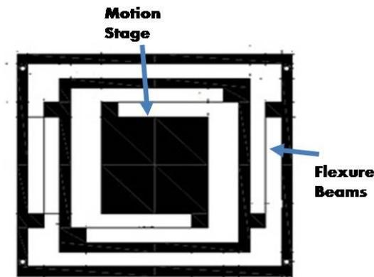
Fig. 5. XY mechanism.
