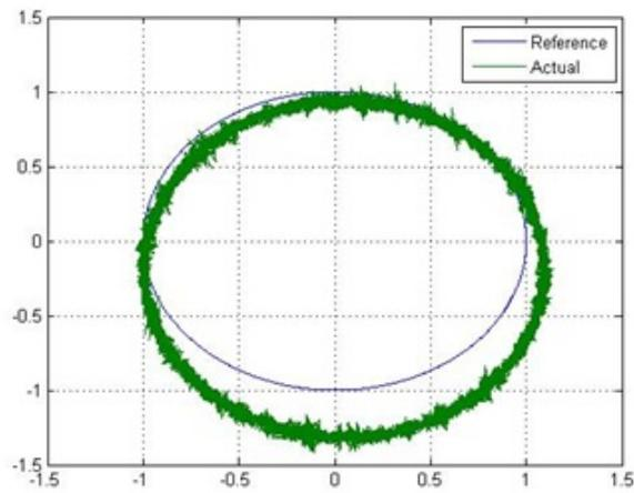
**Fig. 11. Performance of the system when tracking a circle.**
