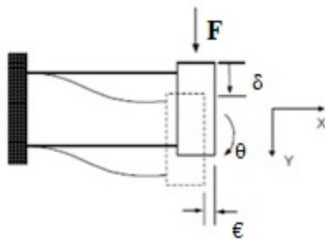
Fig. 3. Parallelogram flexure.
