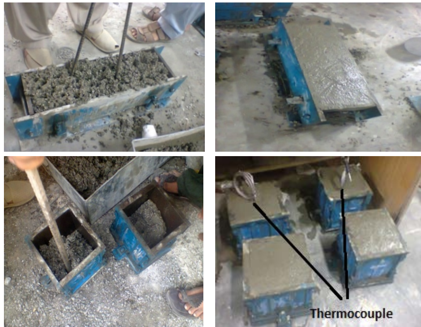
Fig. 5. Moulding of the cubes and prims in the investigation.
