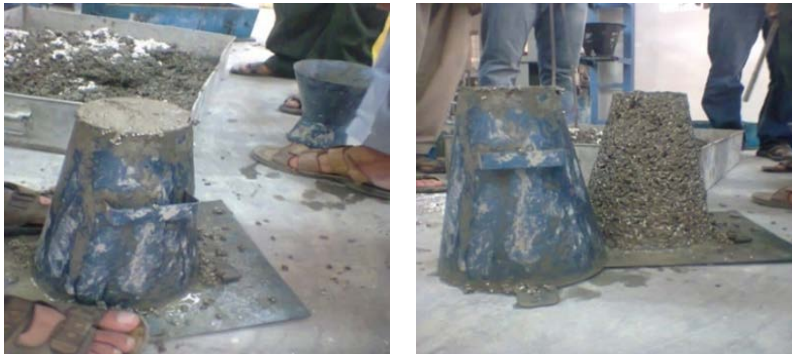
Fig. 6. Workability test of concrete.
