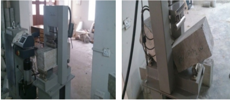
Fig. 10. Flexural strength test on prisms.
