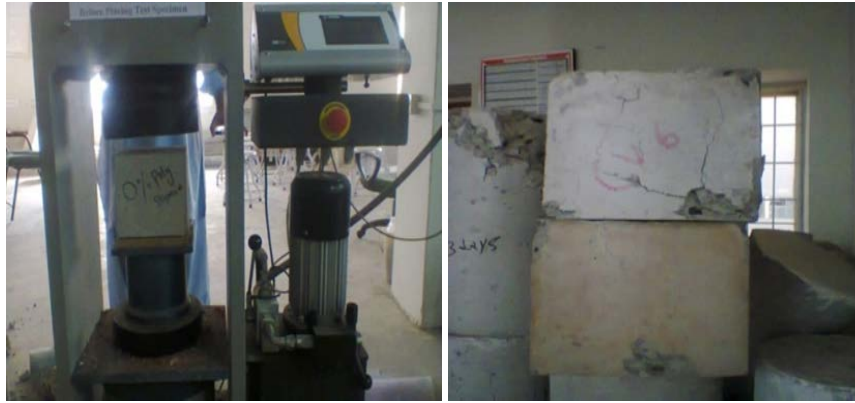
Fig. 8. Compressive strength tests on concrete cubes.
