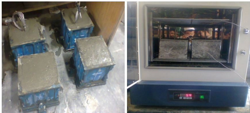
Fig. 14. Performance of the thermal conductivity test on concrete cubes.
