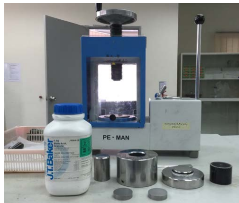
Fig. 4. Hydraulic compacting machine.
