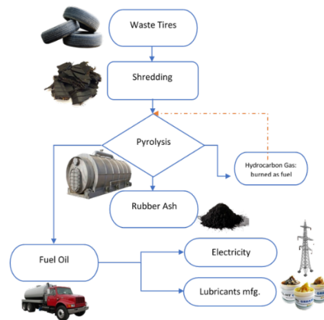
Fig. 1. Pyrolysis process of waste tyre and its by-products (Recycled tyre factory located at Gopeng, Perak, Malaysia).
