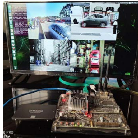
Fig. 7. The hardware implementation of object detection and tracking system.
