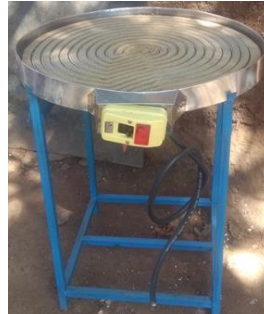
(b). Mitad stand with resistor embedded clay.
