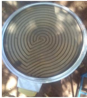
(a). Heating element embedded in clay.
