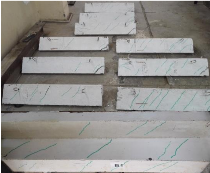
Fig. 5. Failure mode pattern of the RPC beams.
