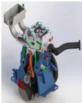
(a) Design of LIPI's range extender engine.
