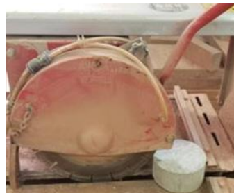
(b) Axially splitting of concrete sample to determine the chloride depth penetration depth.
