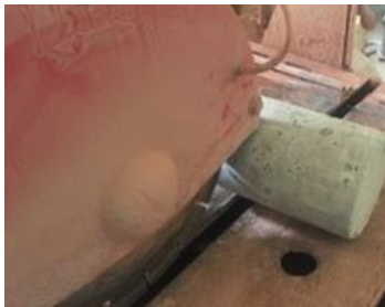
(a) Cutting of 50 mm sample for the RCP test.
