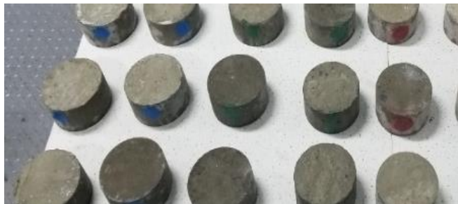
Fig. 1. Concrete samples cut from 400 mm length and 100Ø of concrete cylinder.
