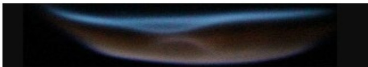
Fig. 10. Experimentally flame front visual data of CH 4 /CO 2 /O 2 with equivalence ratio of 0.90 and flow rate at 6 L/min
