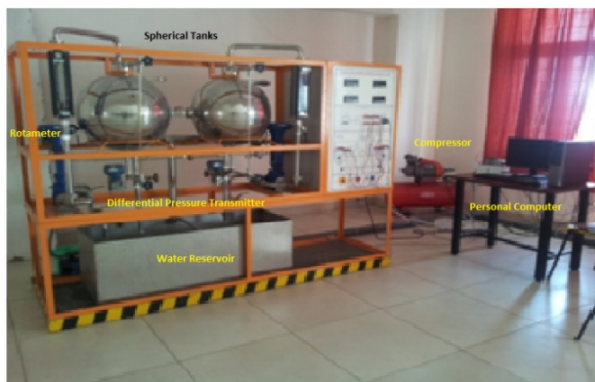
Fig. 1. Real time experimental set up of the DSTLLS process.
