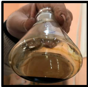
(a) The asphalt content sample was dissolved by adding 1 ml of toluene.
