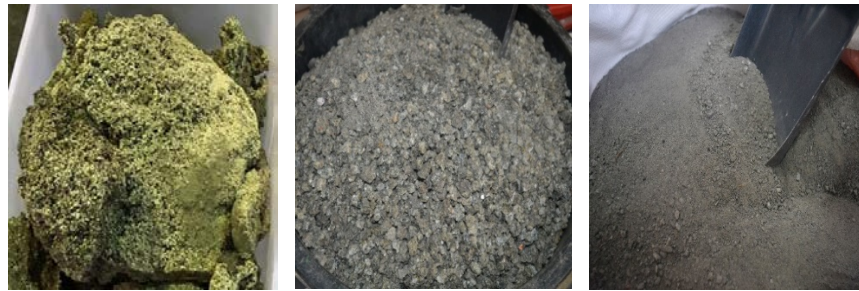
(a) POC raw material. (b) POC coarse aggregate. (c) POC fine aggregate.
