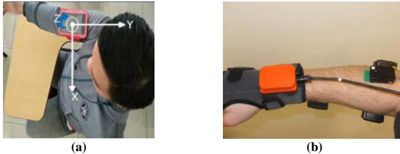
Fig. 1. (a) Related work using sensor in smartphone and jerk of upper arm (top view); (b) Related work using industrial IMU and EMG sensor attached on the forearm.
