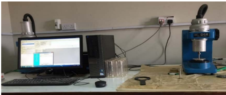
Fig. 2. Testing method of the modified asphalt specimens by the DSR equipment.
