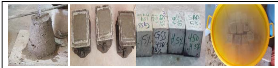
Fig. 2. Preparation of concrete cubes.
