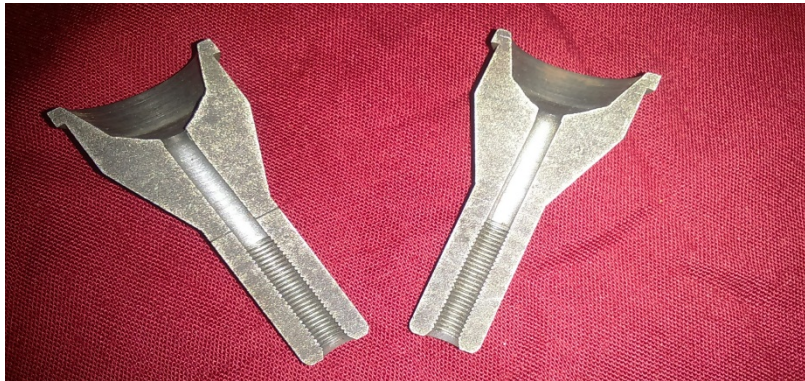
Fig. 1. Cut sectional view of internally threaded nozzle.
