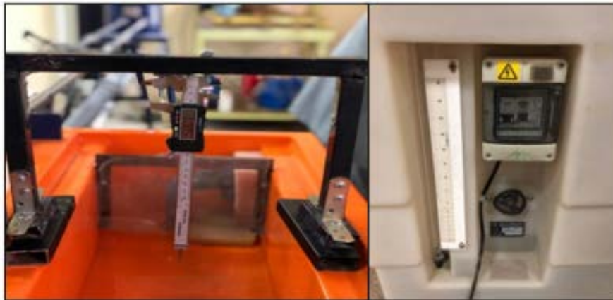
Fig. 2. The laboratory channel and volume measuring tank.
