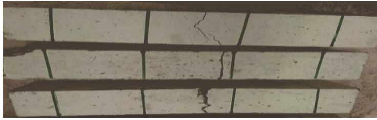
Fig. 12. Failure mode of prisms.
