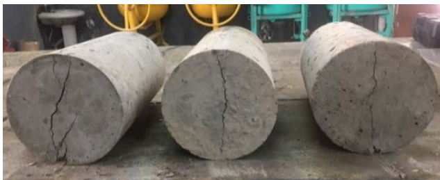
Fig. 11. Failure mode of some cylinder.
