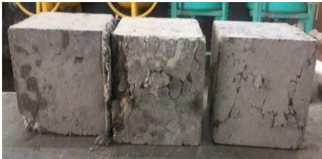
Fig. 10. Failure mode of some cubes.
