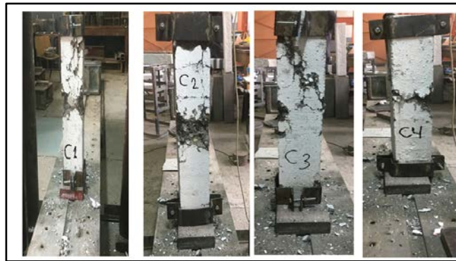
Fig. 13. Mode of failure with conventional crushed for all columns.
