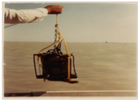
(b) The steal holder and container for collection of composite water samples.
