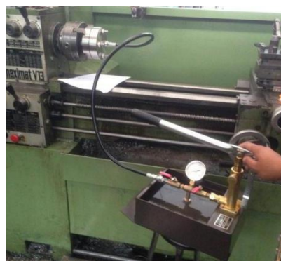
Fig. 9. Experiment setting of the water pressure test.
