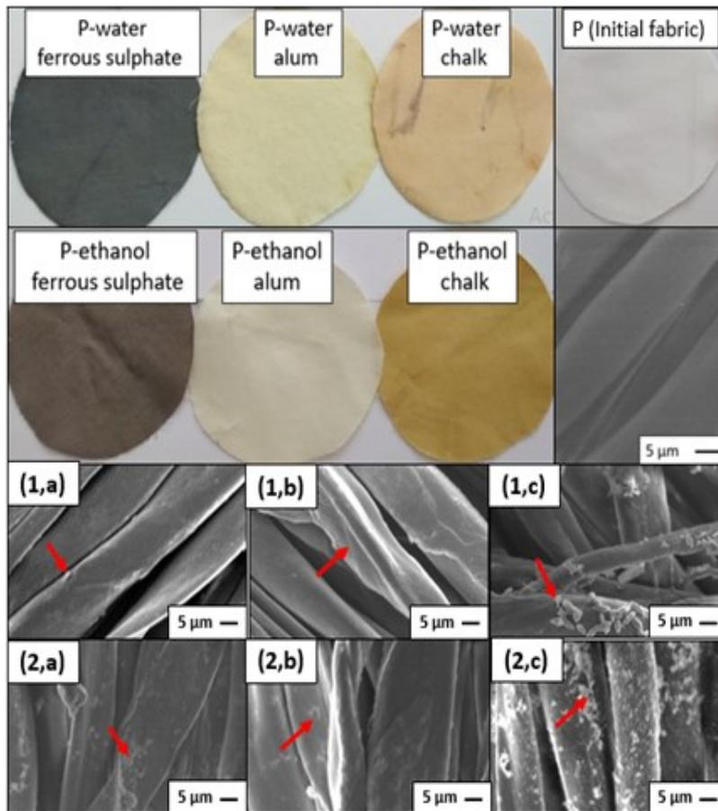
Fig. 6. The photograph images and SEM analysis results of initial fabric of prima and final fabrics of prima coloured by guava leaves extract using (1) water and (2) ethanol as solvents and (a) ferrous sulphate, (b) alum, and (c) chalk as fixation agents.
