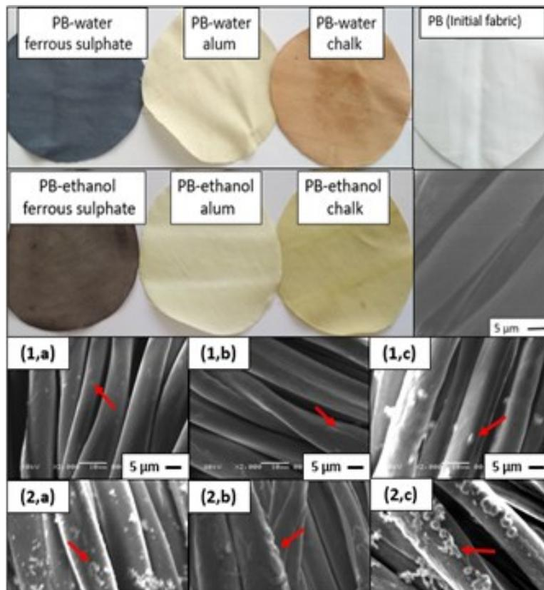
**Fig. 8.** The photograph images and SEM analysis results of initial fabric of primisima B and final fabrics of primisima B coloured by guava leaves extract using (1) water and (2) ethanol as solvents and (a) ferrous sulphate, (b) alum, and (c) chalk as fixation agents.
