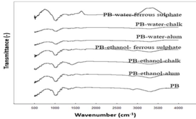
Fig. 5. The results of the FTIR analysis of the primisima B fabric that has been coloured.
