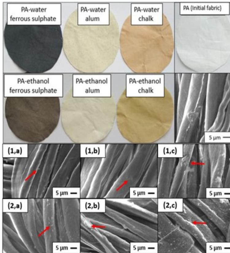
**Fig. 7. The photograph images and SEM analysis results of initial fabric of primisima A and final fabrics of primisima A coloured by guava leaves extract using (1) water and (2) ethanol as solvents and (a) ferrous sulphate, (b) alum, and (c) chalk as fixation agents.**
