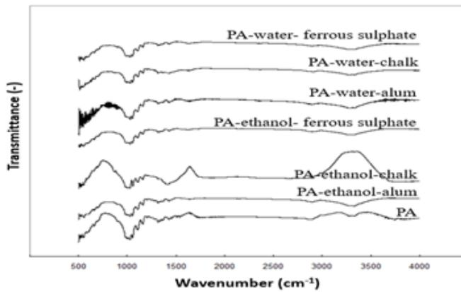
Fig. 4. The results of the FTIR analysis of the primisima A fabric that has been coloured.
