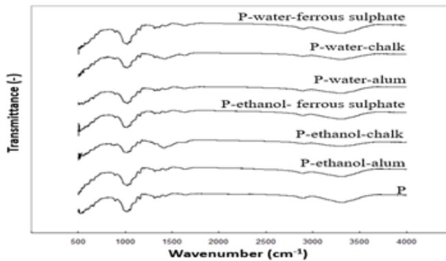
Fig. 3. The results of the FTIR analysis of the prima fabric that has been coloured.
