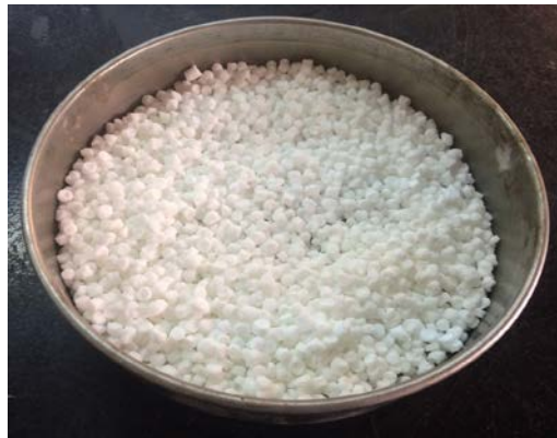
Fig. 2. Forms of the styrene- butadiene- styrene (SBS) polymer.
