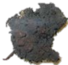
Fig. 4. Peat specimen crusting and burning in microwave oven after 10 minutes.
