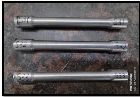
Fig. 3. Round tensile specimens as prepared.
