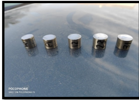
Fig. 4. Prepared specimens for SEM microstructure and EDS tests of (W, S 1 , S 2 , and S 3 ) specimens.
