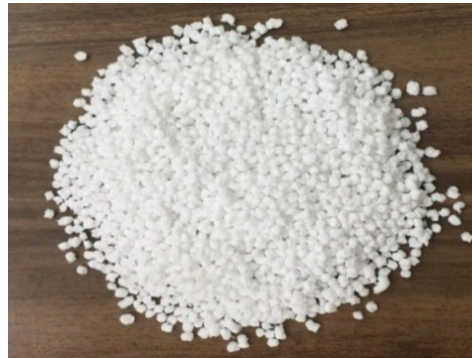
Fig. 4. The photo of SBS used in preparing modified asphalt mixes.
