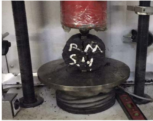
Fig. 5. Specimen tested in ITS device.
