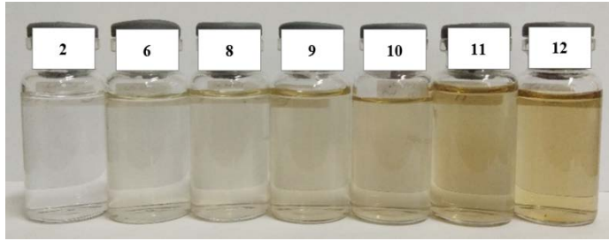
Fig. 3. Photograph image of carbon nanoparticles solution at various pH from 2 to 12.
