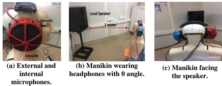
Fig. 3. PNR measurements in an anechoic room.
