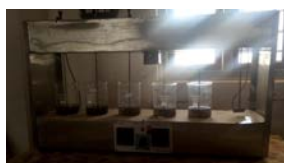
(b) Flocculation coagulation Moringa oleifera seeds powder on wastewater coffee processing (WWCP).
