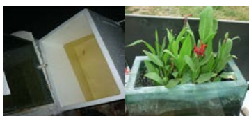
(c) Vertical subsurface flow constructed wetland (VSSFCW).
