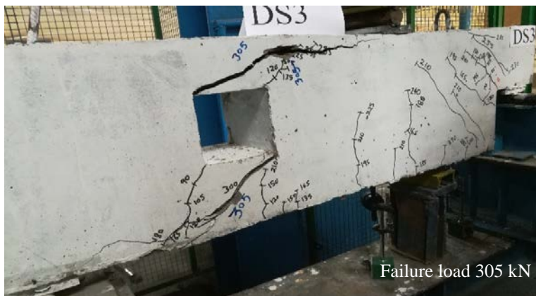
Fig. 14. Crack pattern for specimen DS3.
