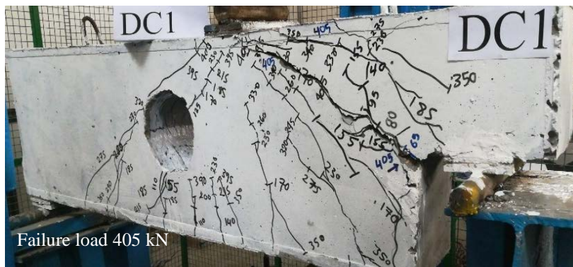
Fig. 9. Crack pattern for specimen DC1.
