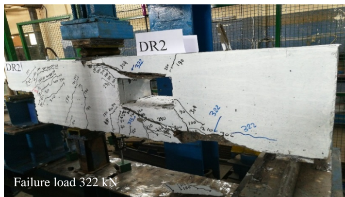
Fig. 16. Crack pattern for specimen DR2.
