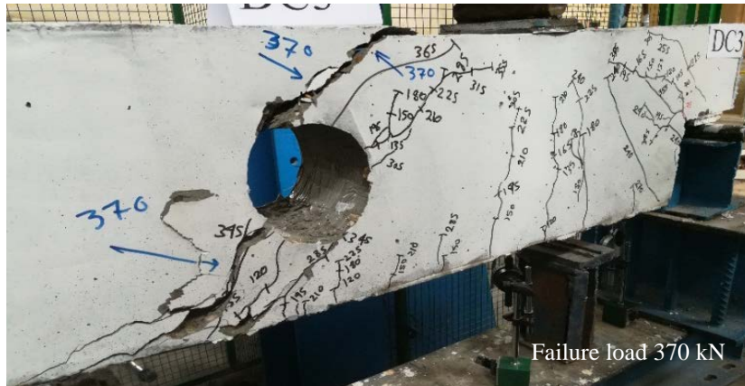
Fig. 12. Crack pattern for specimen DC3.
