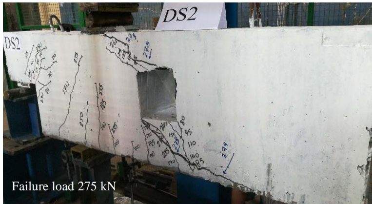
Fig. 13. Crack pattern for specimen DS2.
