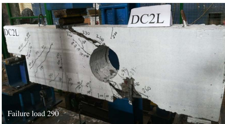
Fig. 15. Crack pattern for specimen DC2L.
