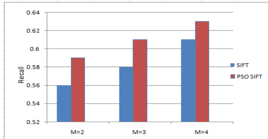
Fig. 6. Variation of recall for different values of M (number of relevant multiple images).
